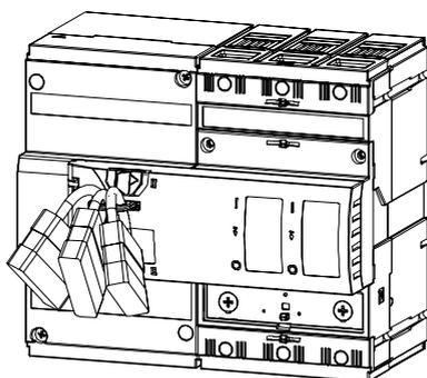
**! Attention!** With locking bar withdrawn the motor drive is disconnected from supply voltage.
