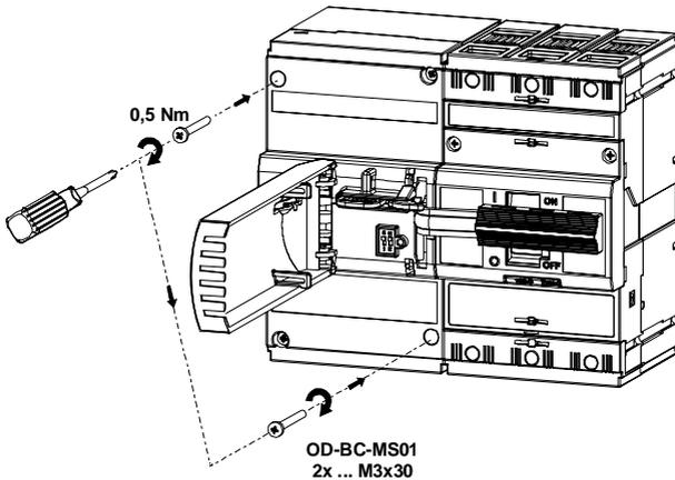
**19** Drive fastening by means of DIN rail
