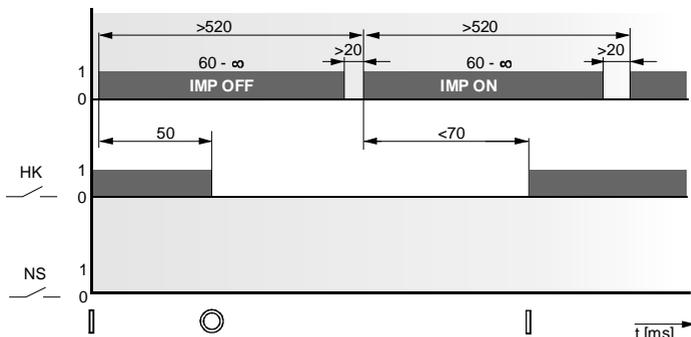
**44** **Circuit breaker switching off by overcurrent release or inspection push-button**
