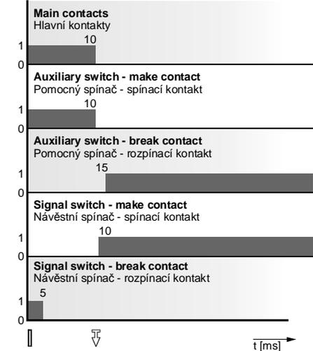
**52** **Recommended control impulses for circuit breaker switching on/off by motor drive after switching off by an overcurrent release or inspection push-button**
